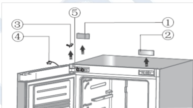
① Upper hinge cover ② Top cover block ③ Left upper hinge cover ④ Display board connecting wire ⑤ Upper hinge part
